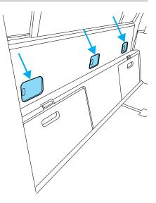
• You may need to pull the seatback forward to access the tether anchors. Make sure the seat is locked in the upright position before installing the child seat. Refer to *Folding Down The Rear Seats* in this chapter for information on how to operate the rear seats.
